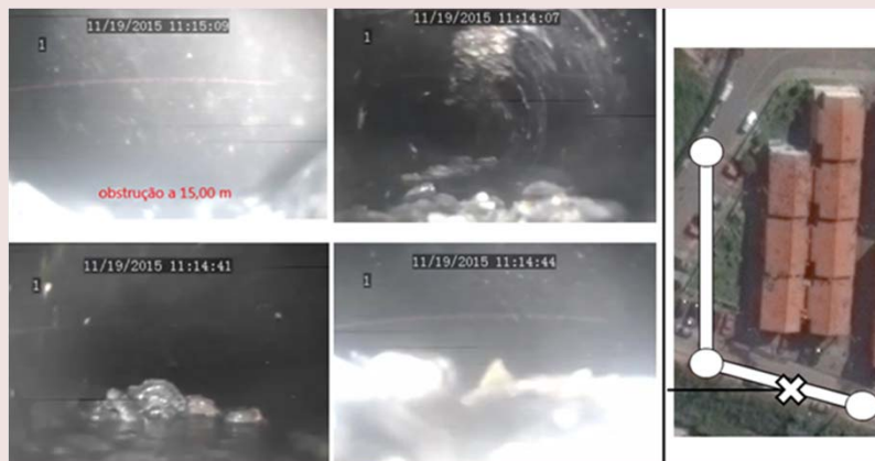
Detail of obstruction noted in real-time video of 11/19/15
