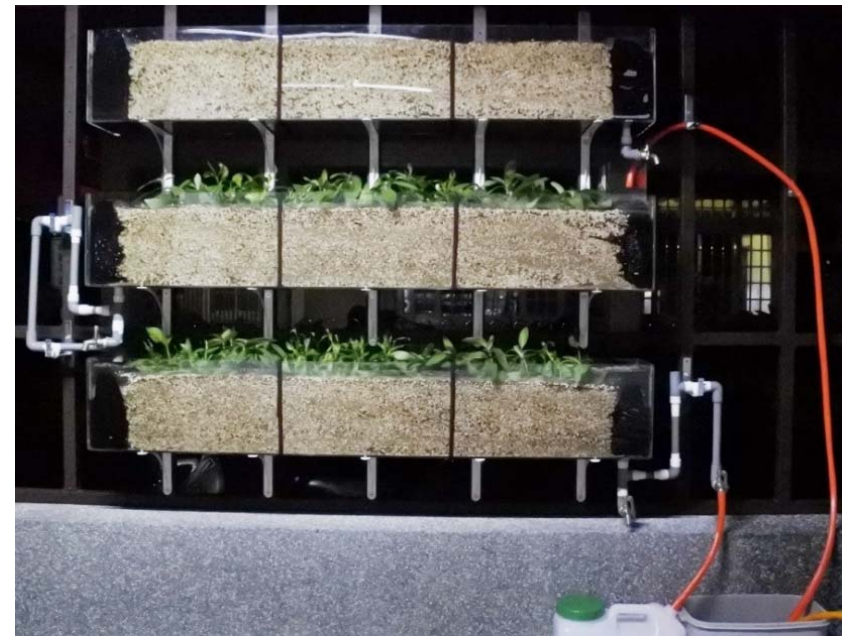
Purification green-wall system (PGWS) established by C.H. Yeh (2016)
