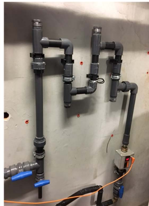
Corrosion racks with hot dipped galvanised steel coupons (UNS G10100 and ASTM D7091)
